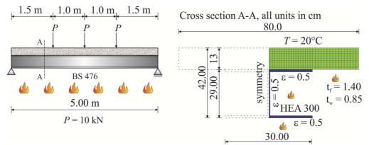
Figure 18: Composite steel-concrete beam
