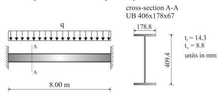
Figure 10: Fully restrained steel beam
