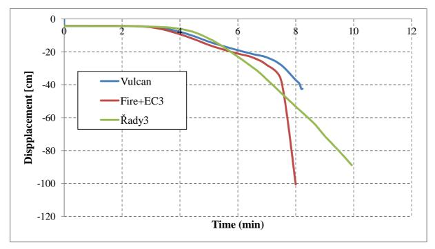
Figure 9: Displacement in the mid-span of the beam, load q = 40kN/m
