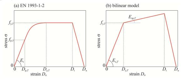
Figure 4: (a) Stress-strain relationship of steel at elevated temperature (EN 1993-1-2, 2005). (b) Bilinear material model of steel.
