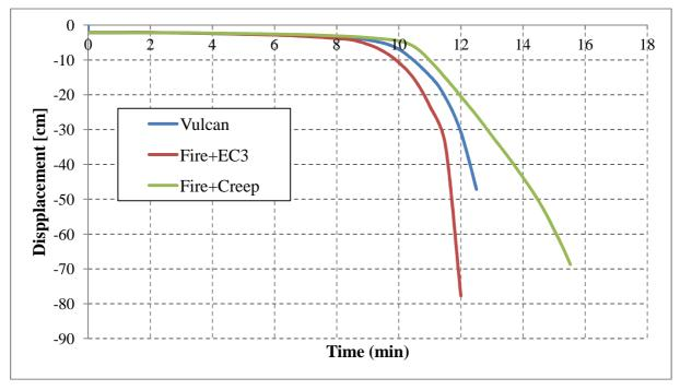
Figure 8: Displacement in the mid-span of the beam, load q = 20kN/m
