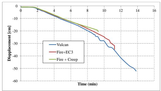
Figure 12: Displacement in the mid-span of the beam, load q = 40kN/m
