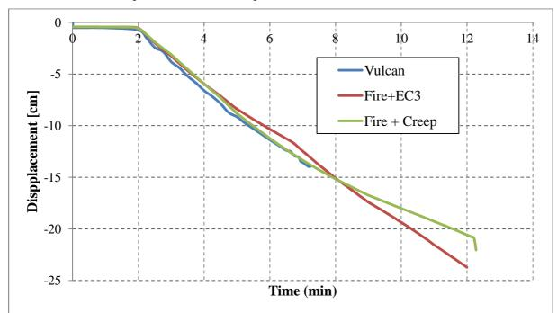
5.2.1. Vertical displacement in the mid-span of the beam
