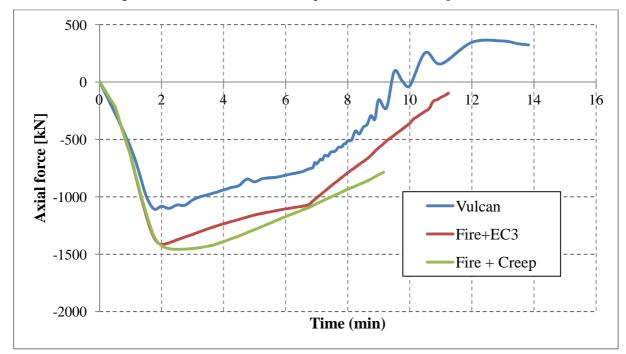
Figure 14: Axial force in the mid-span of the beam, load q = 40 kN/m
