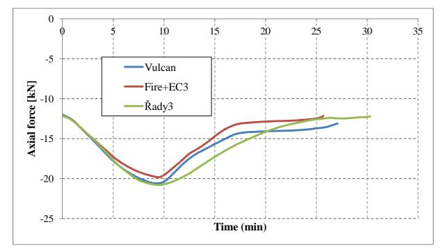
Figure 17: Axial force in the mid-span of the beam, load q = 30 kN/m
