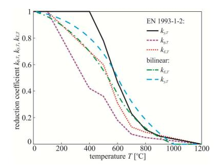
Figure 5: Change of reduction factors with temperature.
