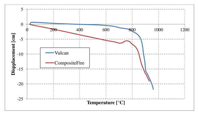
Figure 19: Displacement in the mid-span of the composite beam
