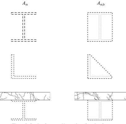
Figure 2: Section factor and box value of section factor
