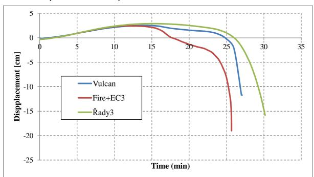
5.3.2. Displacement in the mid-span of the beam
